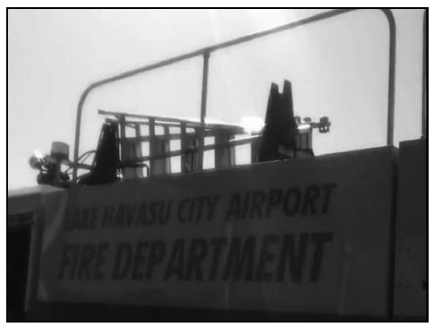
The roof of the apparatus is where a generator is stored, ladders, and a "piercing nozzle" (allows firefighters to spear the aircraft & spray through holes in the end).
