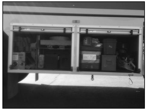
Inch and three-quarter hand-line (shown far left) deploys water. A large array of extrication tools to cut into the side of an aircraft, including a circular saw (shown far right). Hazmat containment equipment.
