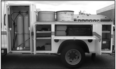
4 air-tank refills (two per side of the truck), Pony Bottles (5 min. "spare air"), wood plugs for plugging up 55 gal. barrel drums and keep them from leaking, "Over Barrels" can hold a 55 gallon barrel inside for containing/sealing the hazard.
