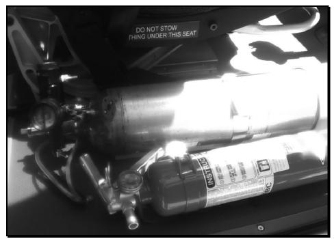
**Fire Extinguisher and Portable Oxygen Tank** – already on the gurney, this one may be used when transporting a patient out of the ER and onto the aircraft.
