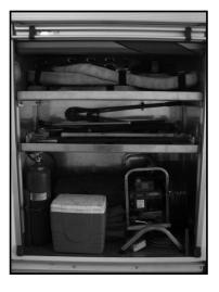
Force Entry Tools The "TNT" Sledge, Sledge Hammer, Electric Fan, and Water
