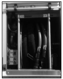
Booster Line – deploys water and foam, controlled by either of the Engineer Panels, or inside of the AARF vehicle.
