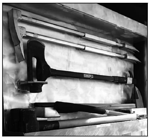
Forcible Entry Tools – Shovels, Axes, Pry Bars, Sledge Hammers
