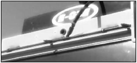
A spray system is also located just above the windshield to allow the apparatus to get in as close as possible to perform a rescue and still keep the vehicle cool.
