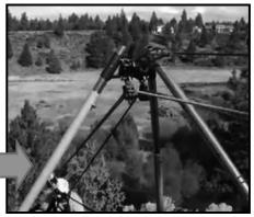
**ARIZONA VORTEXT MULTIPOD** Designed by a TRT Firemen here in Arizona, provides a portable base for rescuers to rappel.
