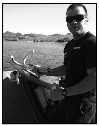
This grappling hook, attached to the fireboat, is used to keep a burning boat a set distance from the fireboat, as well as keeps it from pushing away from them as they fight the fire.
