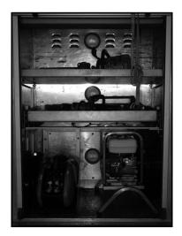
Gas Powered Tools Compartment Chainsaw, Jaws of Life, Fan Supply/Working Hose (top-out of view)
